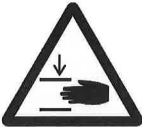
Figure 3-6: Label „Danger of get one's hand crushed" while closing chamber door
