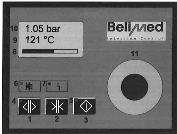
Figure 4-7: Non operating end control panel
